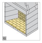
Cut 50mm thick fire-bricks and glue to the back of firechest with fire-brick mortar.
