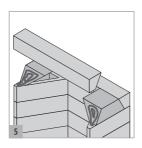
Bed the first layer of Gather as above using beads of lip glue. Check it is plumb and level.
