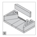
Bed the first back element using lip glue beads as shown above. Lip glue joints should be 2-3mm thick, wipe away any excess.
