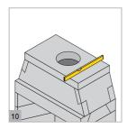
Bed on the top plate slab. Check all plumb and level, remove any excess glue.
