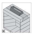
Fit the damper loose onto the gather elements. No mortar or lip glue is used to fit the damper.
