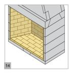
Point in the fire-bricks with the fire-brick mortar and wipe away excess.
