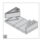
Mix the lip glue as per instructions on bag. Using the supplied application bag bed the first 2 side elements using lip glue beads as shown above.
