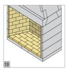
Cut 25mm thick fire-bricks and glue to the sides of firechest with fire-brick mortar.
