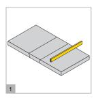
Bed base slabs onto a suitable foundation using mortar. Check it is plumb and level.
