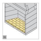
Cut 50mm thick fire-bricks and lay loose on the base. Glue the front row of bricks with fire-brick mortar as per the instructions on the bag.
