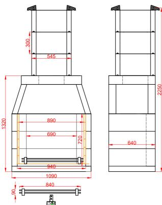
We recommend a minimum 100mm thick reinforced concrete slab to bed the garden fireplace onto, size should be at least 150mm wider than the Garden fire on all 4 sides
