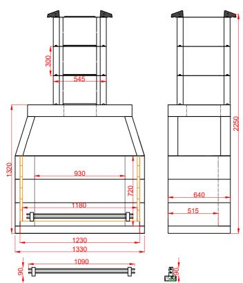
We recommend a minimum 100mm thick reinforced concrete slab to bed the garden fireplace onto, size should be at least 150mm wider than the Garden fire on all 4 sides
