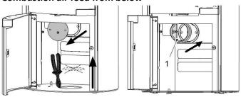
1.) Carefully remove the bottom supply air cover using cutting pliers. Then screw off the inner lid.
