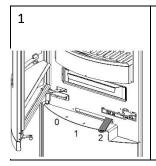
To start the heating process, move the combustion air regulator above the combustion room door onto "Ignite".
