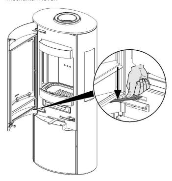
**Warning!** Never leave the door in the secured open position during heating.
