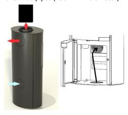
Combustion air comes from the room where the device has been installed (not recommended by SCHIEDEL) (changing to this variant as described in related paragraph – combustion air feed from below)
