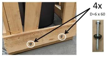
To remove the wooden crate, four screws have to be removed (on each corner one).
