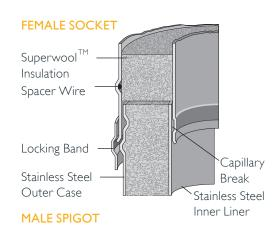
Sleeve joint with locking band for:
