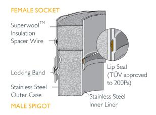
Sleeve joint with integral lip seal on the liner and locking band for:
