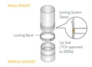
Sleeve joint with lip seal and locking band for:
