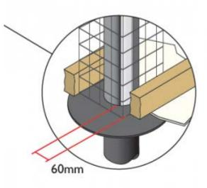
From the image, you can see the distance in a bungalow. You can clearly see that the pipe gives 60mm distance between it and the wooden beams
