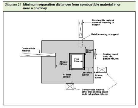
Doc J of Building Regulations shows a diagram in regards to minimum separation distances from combustible material in or near a chimney
