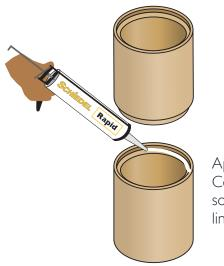
Apply Schiedel Rapid Cement into the socket of the flue liner as shown.
