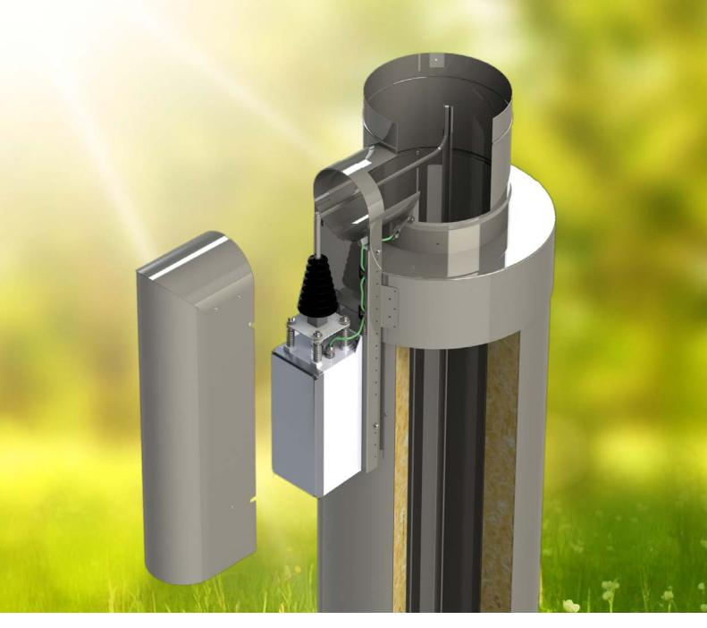
Schiedel ePURO is the fine dust filter for wood burning appliances. It's electrostatic fine dust separator effectively reduces flue gas particles up to 95%.
